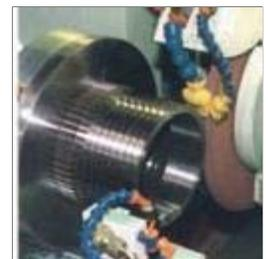
This formed wheel is used to grind semicircular grooves in the winch drum. In this case, the gear
