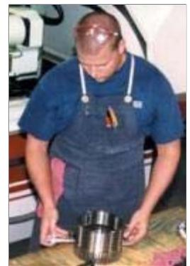
The grinding foreman at Gear Manufacturing, Inc. checks the diameter of one of the grooves on a winch drum, ground on the firm's Studer S30 CNC OD/ID grinder.
