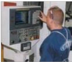
GMI's Tag 400 CNC eight-axis gear grinder, originally purchased to supplement the firm's four older gear grinder, tool over most of the work from those machines. It currently handles 60 to 70 percent of the company's gear grinding.
