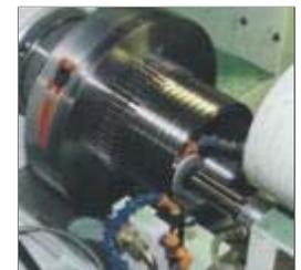
The CNC grinder's turret indexes a second time to present the ID grinding wheel to the winch drum bore. Before advancing to the part, the wheel is dressed by the single point diamond dresser in the foreground.
